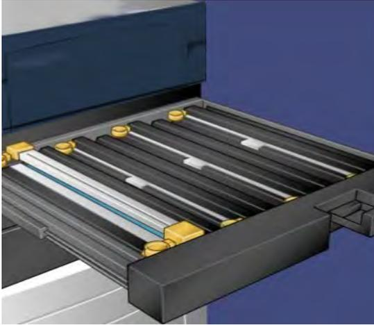
8. Remove the old drum cartridge by holding the finger rings provided at the both ends of the drum cartridge and gently lifting up.
