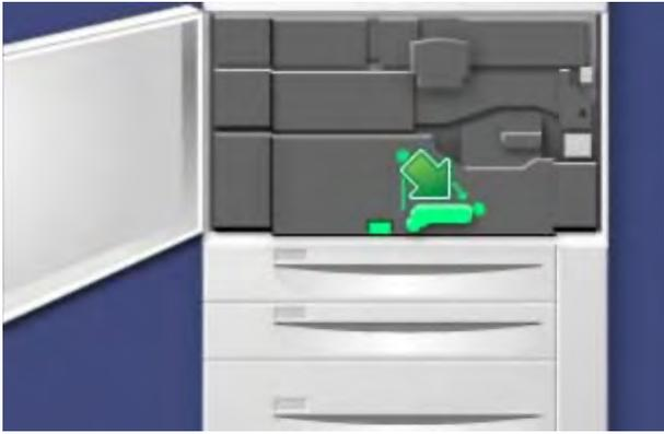
3. Carefully pull out the transfer module.
